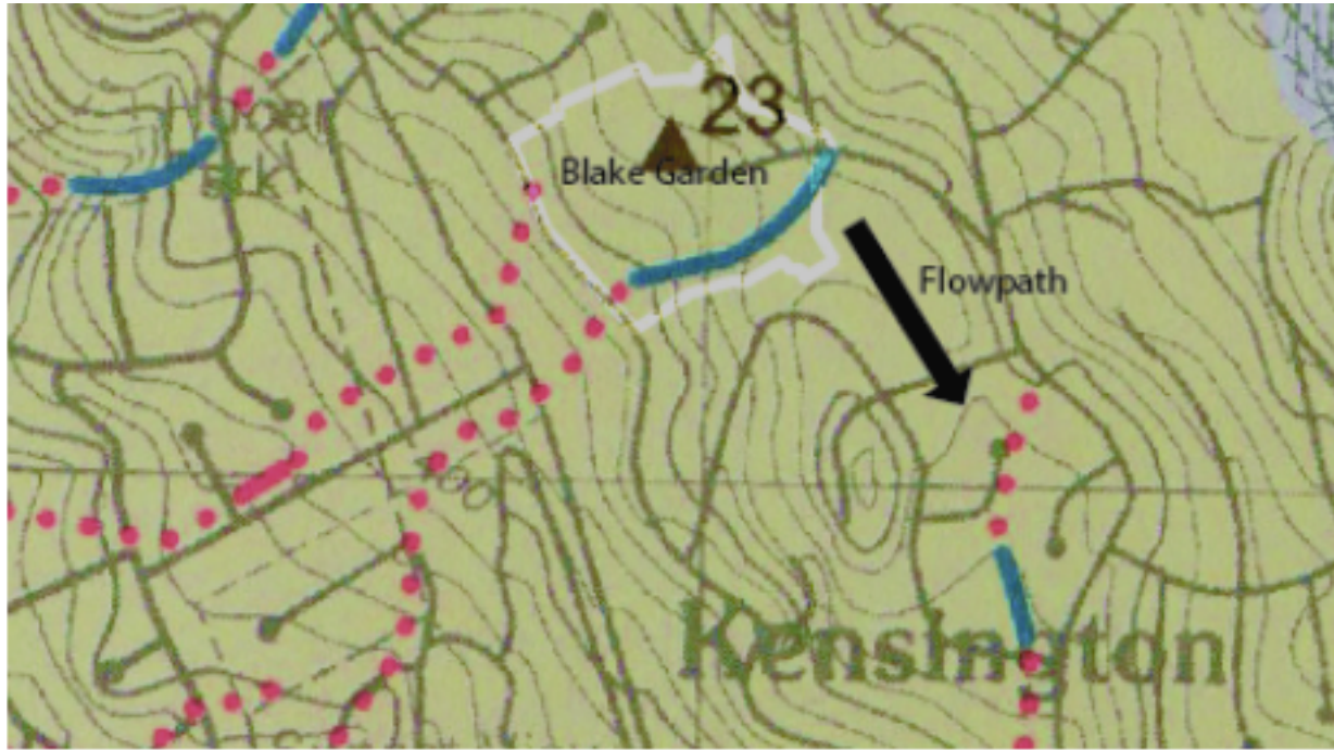
Figure 16. Potential flowpath between floodplain and lower branch of Cerrito Creek.
