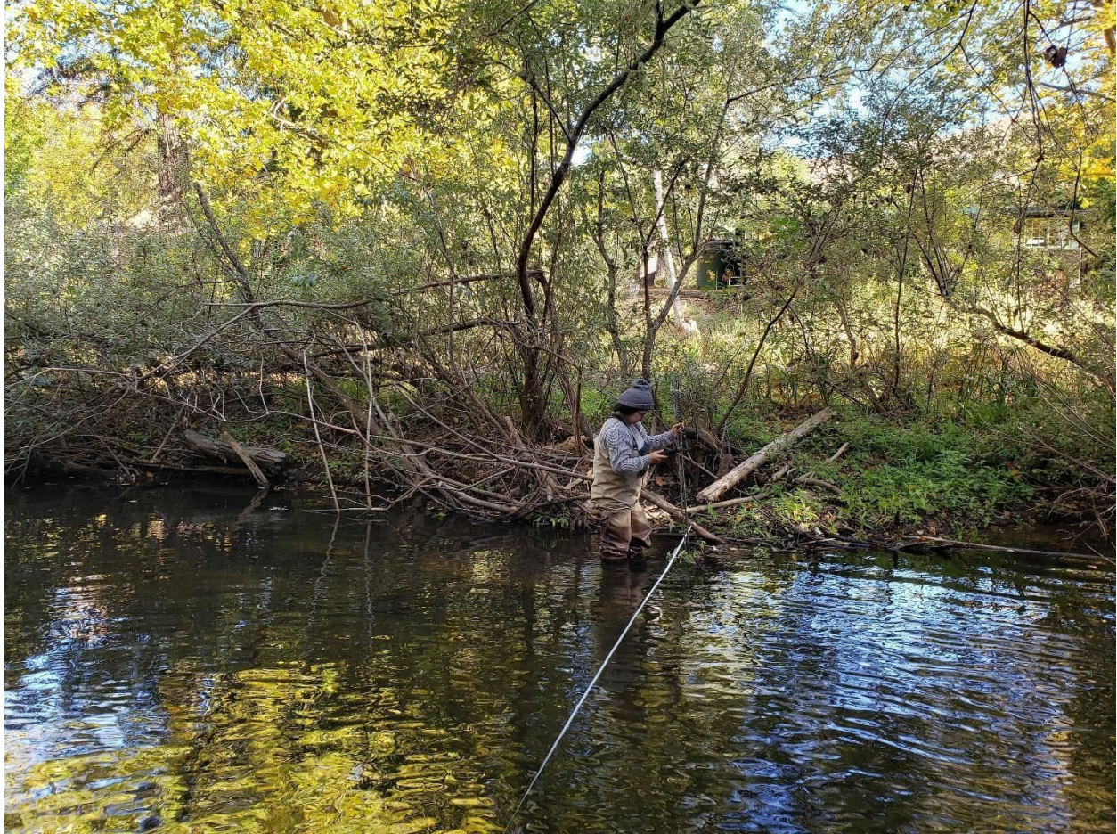
Figure 7: Velocity measurement in the main channel. Velocity measured at discharge of 8cfs on 10/20/19.
