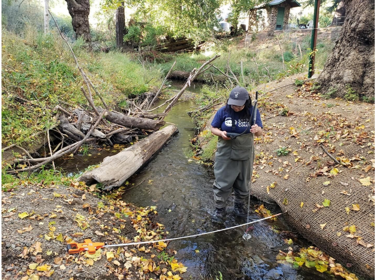
Figure 6: Velocity measurement across the side channel. Looking downstream of side channel.
