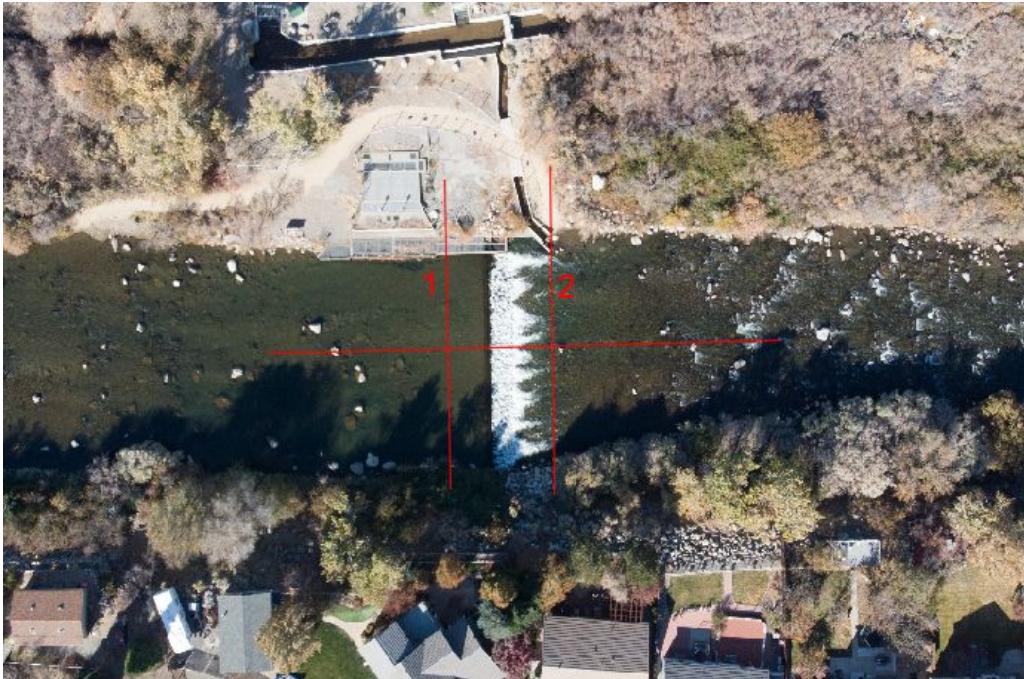
Figure 8: Map of the reference dam site three miles upstream showing cross sections and longitudinal profile surveyed. Imagery from a drone flight during our site visit.
