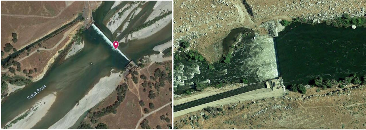
Figure 3: Two examples of diversion low-head dams in CA. Left: Diversion for irrigation. Right: Diversion for small hydroelectric.
