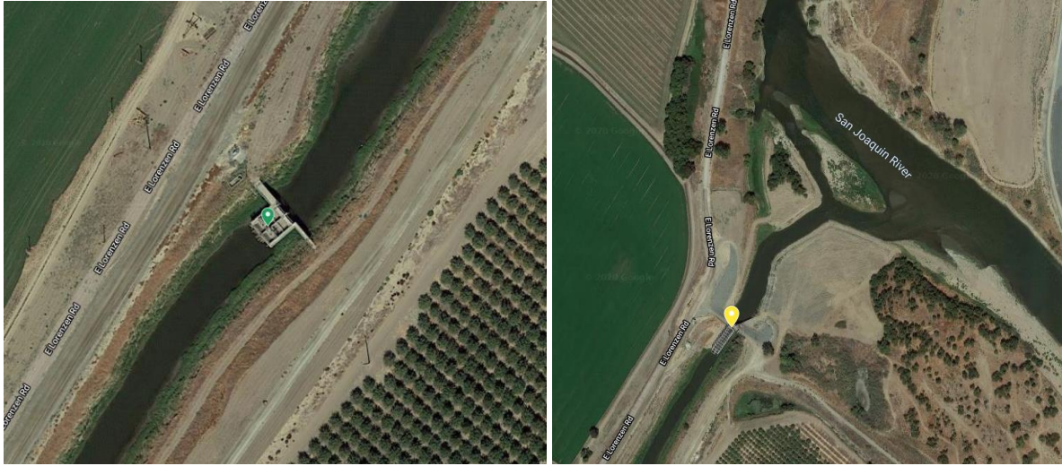
Figure 5: Two examples of low-head dams in irrigation channels.
